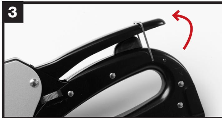
When the handle is fully lowered and resting on the rubber handle stop, secure the handle with the handle loop, as shown above.
