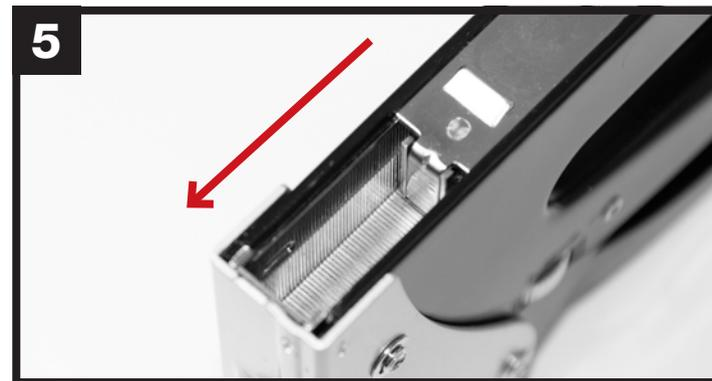
Once correctly positioned, you can close the tacker push bar. If the push bar does not move past the staples, check the position of the staples (steps 3 & 4) and try again.
