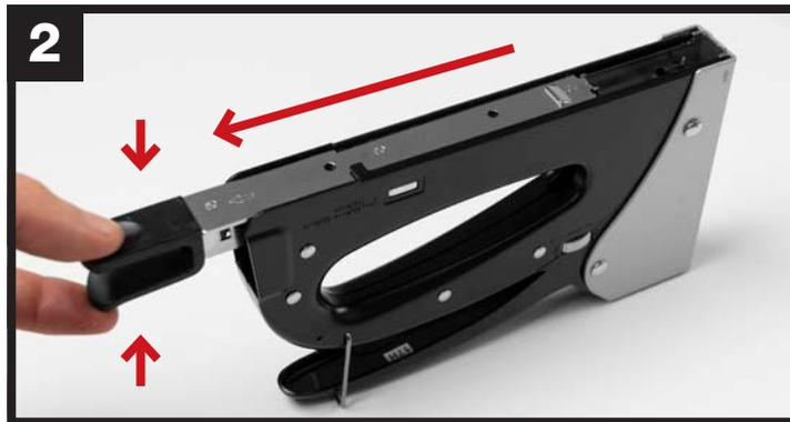
With the tacker turned upside down, pinch the two clips located at the back of the tacker (black plastic) and fully pull the bar outwards to reveal the staple loading trough.
