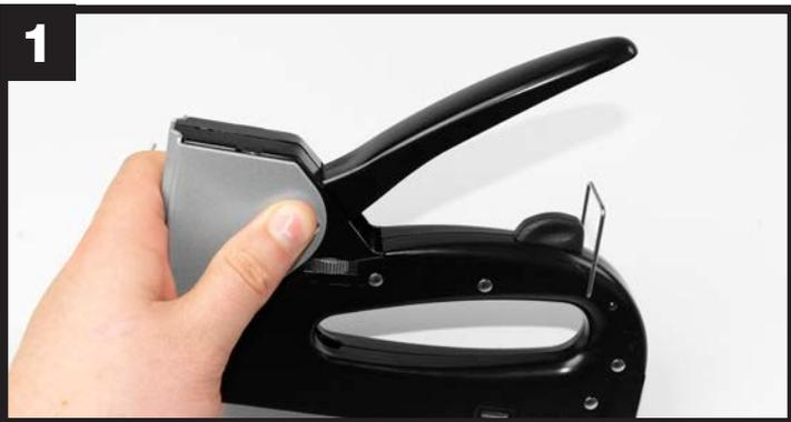
To lock the handle down, you should hold the tacker by the light grey header and ensure the bottom of the tacker is facing the floor away from your body and any other persons.
