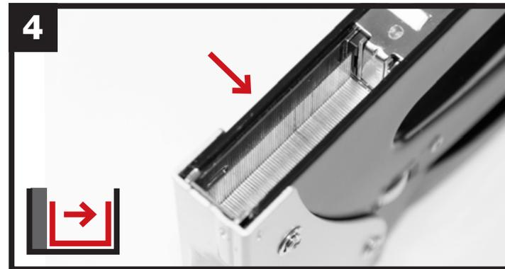
With the front of the tacker (light grey header) facing you, the staples should be on the right-hand side, as shown above. The loading push bar will not close if incorrectly positioned.
