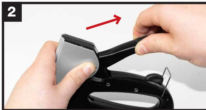
While holding the header firmly, pull the handle outwards. If done correctly, the handle will now feel loose and can be safely lowered towards the body of the tacker.
